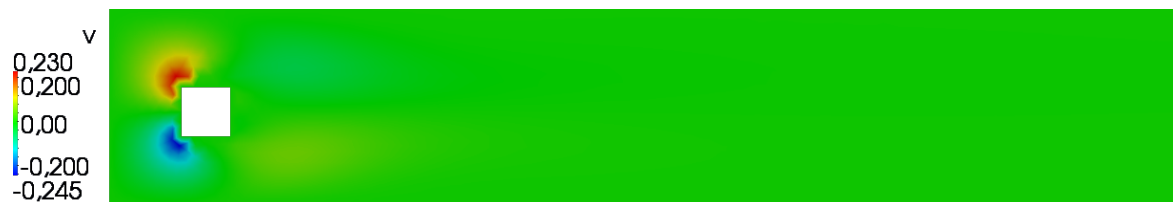
Figure 5: Solution for the u_2 -component (vertical) of the velocity field.
